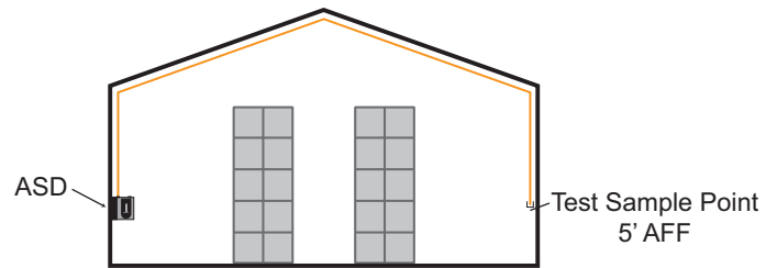
Figure 9. 3-Test sample point for warehouse installation
